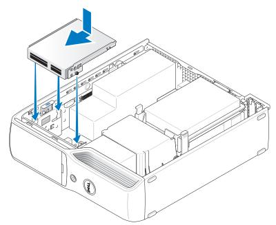
Connect the interface cable to the back of the Media Card Reader and to the Media Card Reader connector on the system board.
