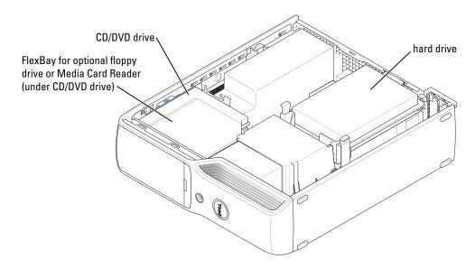
Connect a CD or DVD drive to the connector labeled "IDE OPT" on the system board. A serial ATA hard drive should be connected to the connector labeled "SATA0" on the system board.
