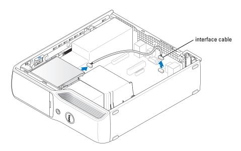
**5** Pull up on the drive release latch and slide the Media Card Reader towards the back of the computer. Then, lift to remove the drive from the computer.
