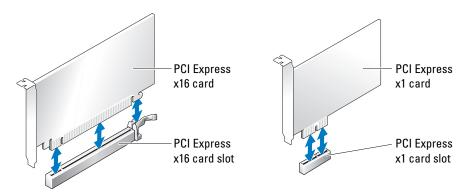
If you are installing or replacing a PCI Express card, follow the procedures in the next section. If you are removing but not replacing a card, see "Removing a PCI Express Card" on page 72. If you are replacing a card, remove the current driver for the card from the operating system.
