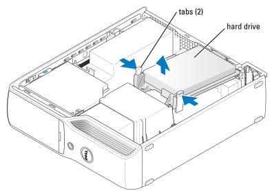
**3** Disconnect the power and hard-drive cable from the drive.
