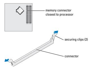
**5** Align the notch on the bottom of the module with the crossbar in the connector.
